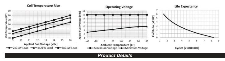
ELO Electronic Flasher w/ Lamp Outage Detection carries  $4 \times 21W + 3W$  on directional lights, and  $10 \times 21W + 2 \times 3W$  on hazard lights. It is designed for vehicles with seperate pilot lamp for each direction (double pilot lamp). If one of the bulbs are malfunctioning or in case of a bulb lower than 21W, the flasher has the ability to warn the driver with an increased speed while functioning. All 3 Terminals of the flasher (+, L, -) are 6,3 mm. plug-in terminals.
